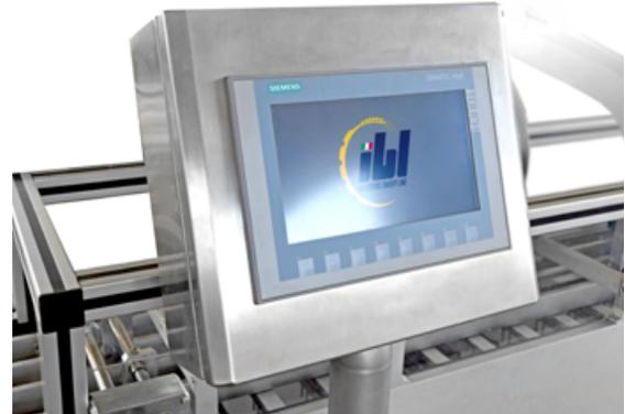
The practical panel allows to optimize the production by the regulation of weight and amount of cream depending on the size of the biscuit and the speed of production.
